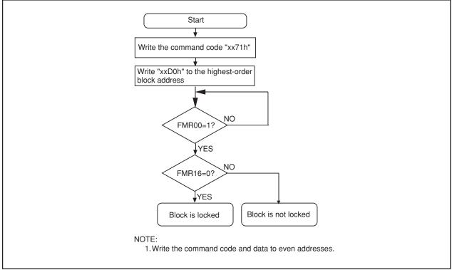
Figure 20.11 Read Lock Bit Status Command
